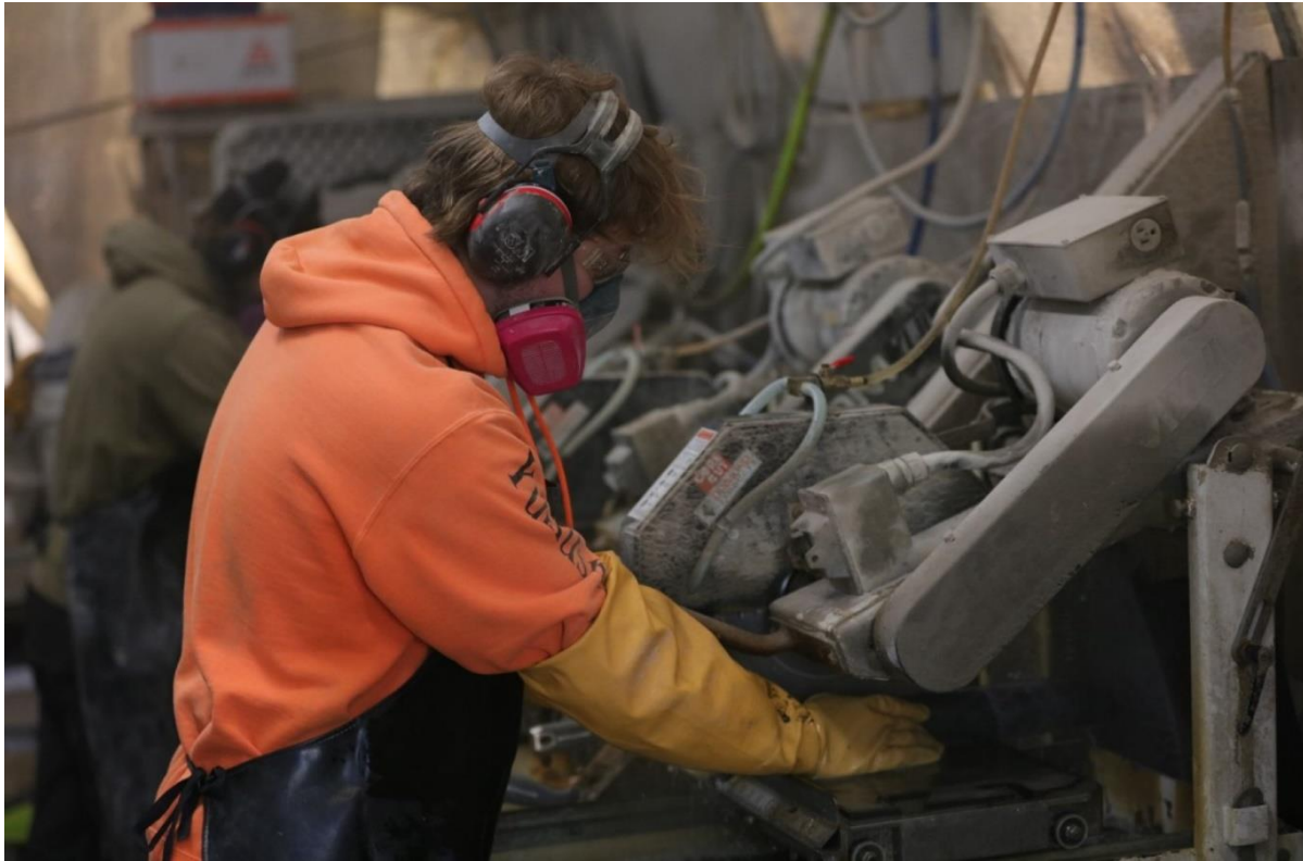
Figure 8-1: Splitting drill core at the Estelle Gold Project
